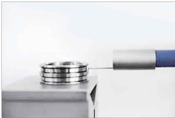
测量轴承挡边粗糙度 Surface roughness measurement of bearing rib
