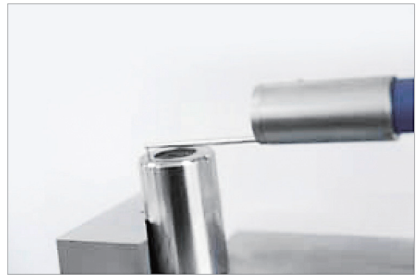
测量轴承滚针端面轮廓 Measuriement of the shape of bearing needle roller end
