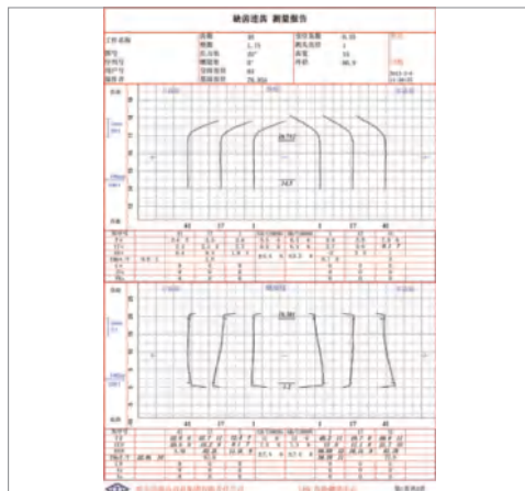
缺齿联齿齿轮齿廓与螺旋线偏差测量报告单 Tooth profile and helix deviation measurement report of the Missing and uncut tooth gear
