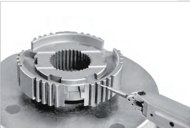
缺齿联齿齿轮测量 Missing and uncut tooth gear
