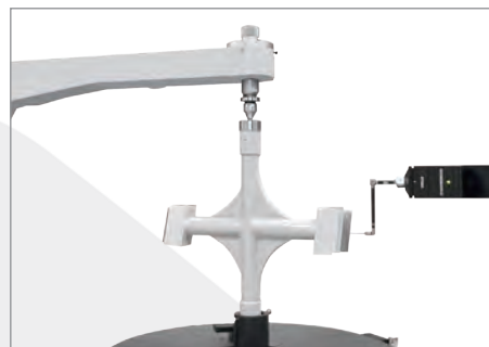
测量样板 Checking the involute
