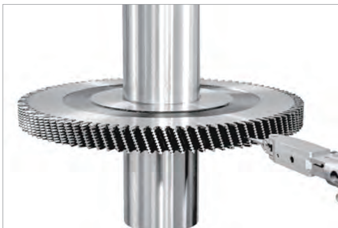
剃齿刀测量 Shaving cutter
