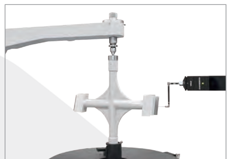
测量样板 Checking the involute
